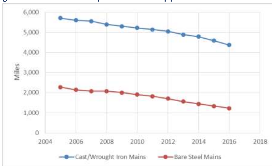
Figure IV.F.-1: Miles of leak prone distribution pipelines located in New Jersey.
